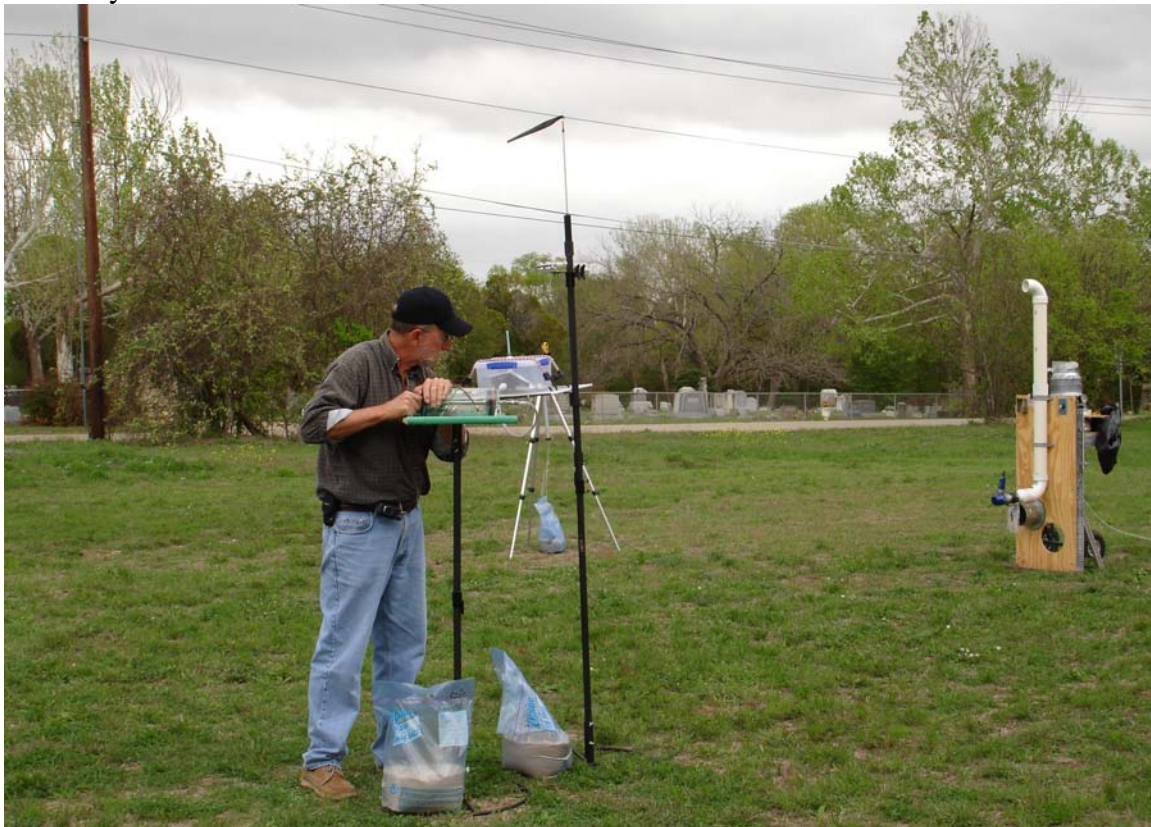
Figure 1: Transient odor event peak sampler process. To the right is the left-most generator configured for controlled emission of the naphthalene / chloroform odorant / tracer pair. The first author is shown awaiting the characteristic sensory cue for the targeted transient event. Utilizing the 1 L manual gas tight syringe, the 1 L m-FEP gas sampling bags could be completely filled in 1-2 sec during the sensory cued events.
