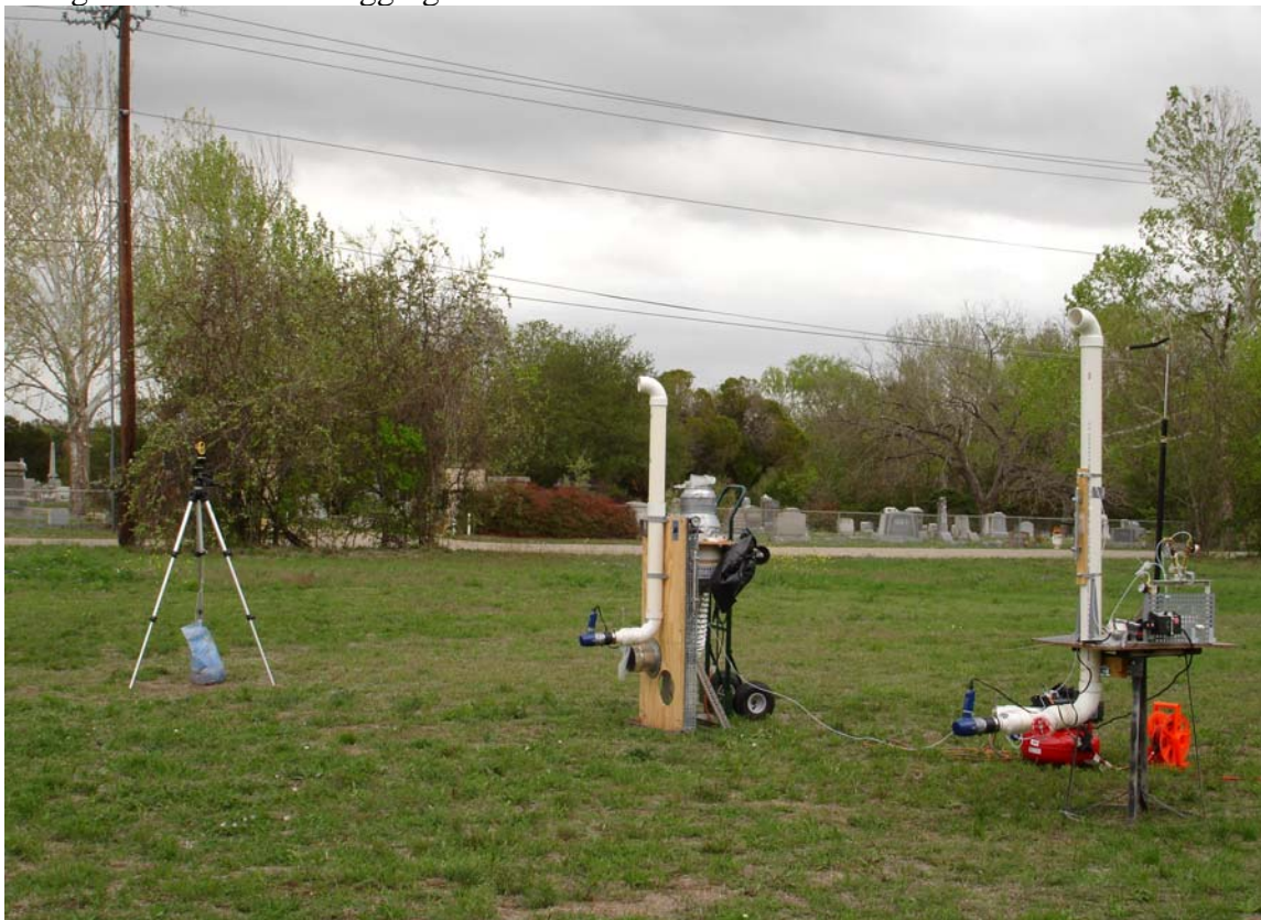
Figure 2: Integrated multiple point-source transient odor event generator system. To the right are the two ‘discrete’ point-sources. to the left background is the tripod mounted weather data logger.
