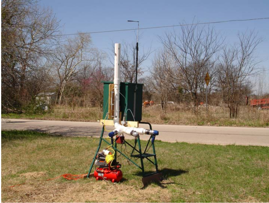
Figure 4 – Prototype scale model transient downwind odor event simulator
